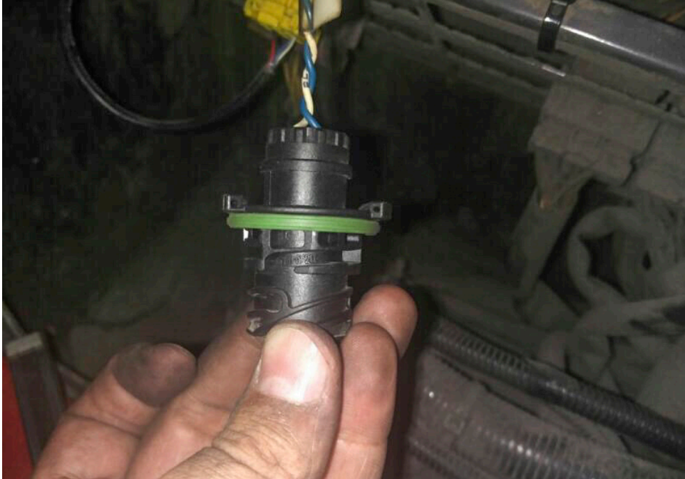
Figure 4. The connection to C471 connector using part No. 1-1719434-1 socket
