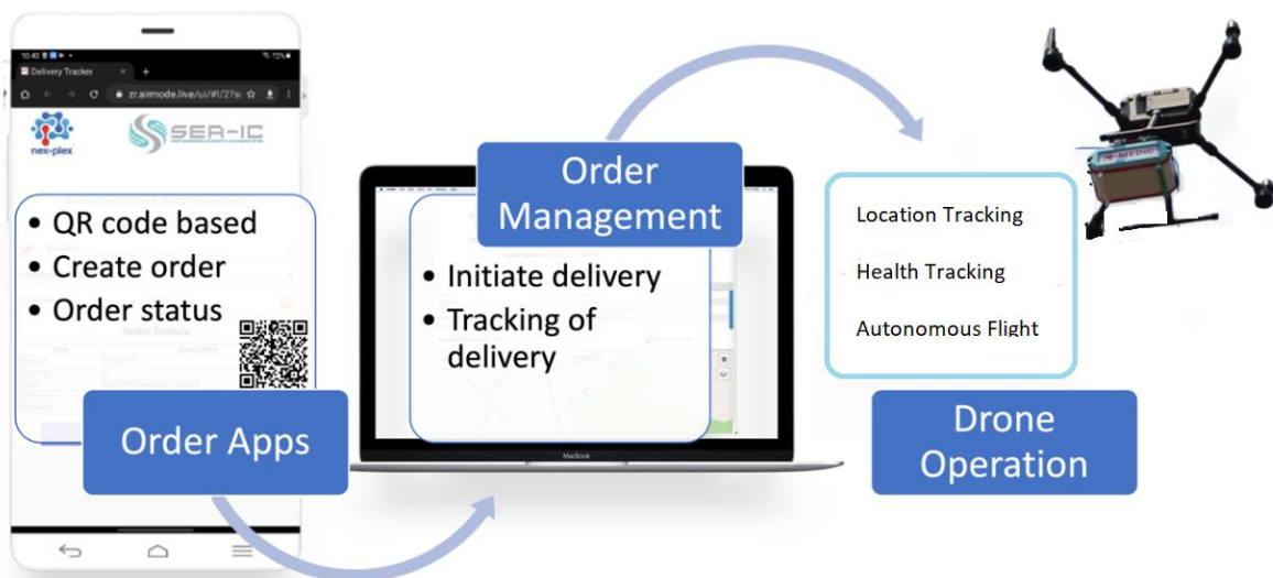
Figure 8. System architecture of drone-based vaccine delivery
