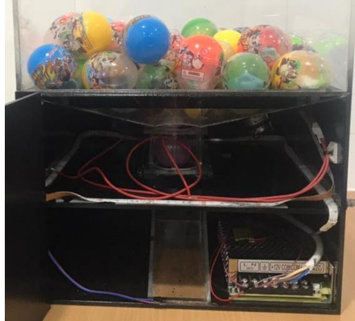
Figure 5. Prototype of reward dispenser
