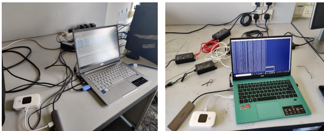
Figure 17. Client (left) and server (right) laptops iPerf3 configuration
