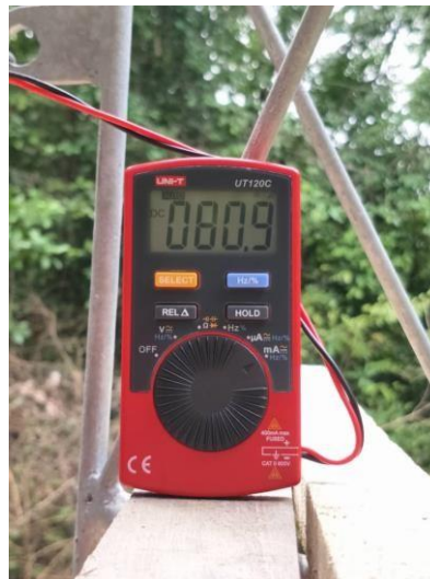
Figure 23. Measurement of power consumption in idle state
