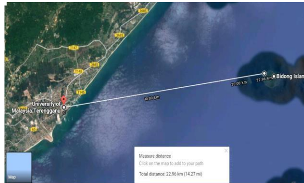
Figure 1a. Project location covers with 23 km line-of-sight radio link from Universiti Malaysia Terengganu (UMT) and Bidong Island, Terengganu
