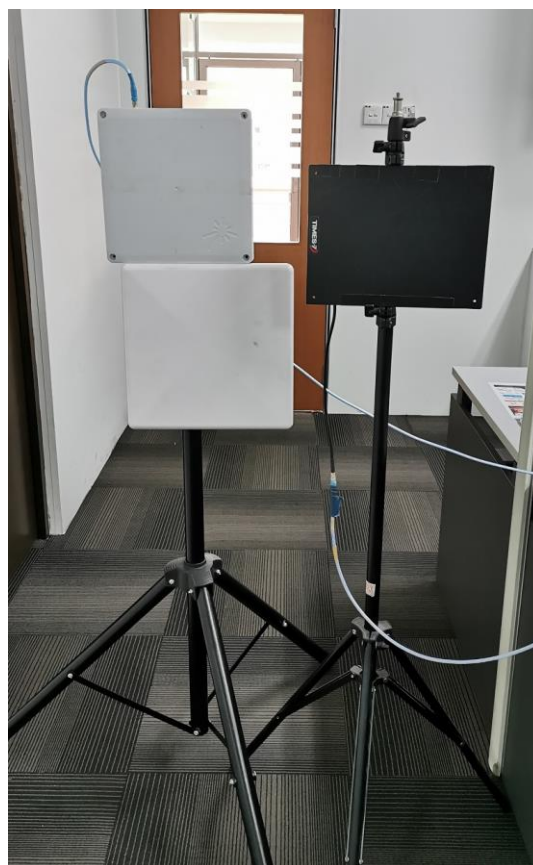
Figure 8: Three antenna for the RFID reader (920 MHz), 920 MHz and 2.45 GHz wireless energy transmitter.
