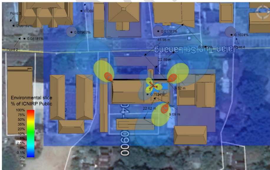
Figure 5: Power density at 2m above the ground level (Top View 2D Elevation)
