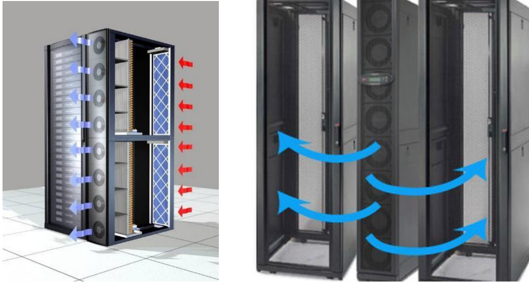
Figure 10.18 Diagram of air-flow from an In Row air-conditioner
