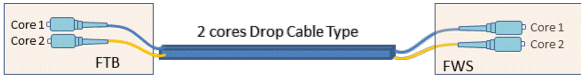
Figure 68. Colour code for 2 cores of drop cable
