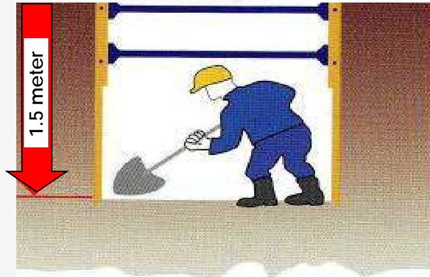
Deeper trench must be shored
