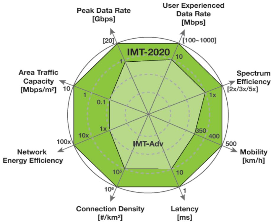
Figure 6: Enhancement of key capabilities from IMT-Advanced to IMT-2020
